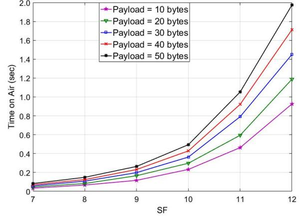
Fig. 8. LoRa<sup>TM</sup> packet time on air with  $BW = 125 \text{ kHz}$  and  $CR = 0$
