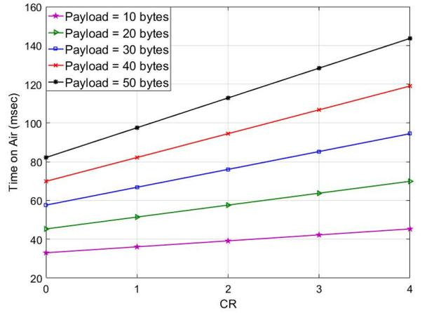
Fig. 9. LoRa<sup>TM</sup> packet time on air with  $BW = 125 \text{ kHz}$  and  $SF = 7$
