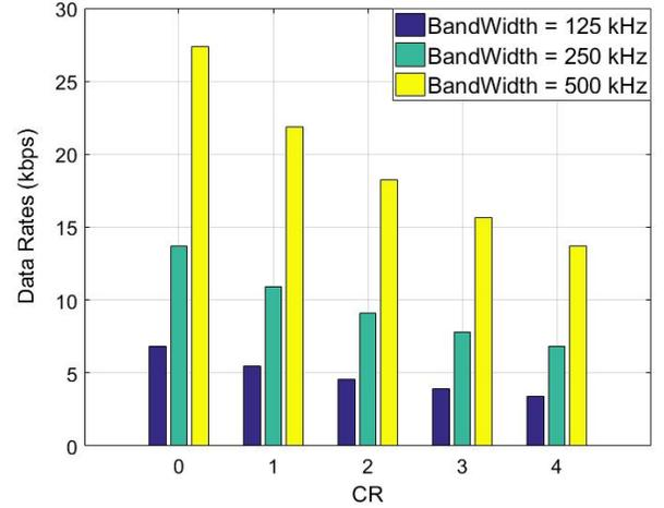
Fig. 3. Data Rates offered in LoRa with different code rate and bandwidth values, ( $SF = 7$ ).
