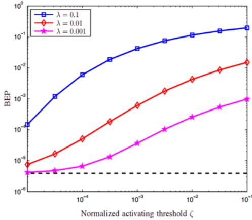
**Figure 5:** Unified BEP of BPSK as a function of the normalized activating threshold  $\zeta$  for the single-threshold protocol.  $E_b/N_0 = 10 \text{ dB}$  and  $SIR = 10 \text{ dB}$ . For comparison, the BEP in the without interference is also plotted (dashed line).
