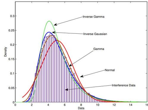
**Figure 7:** Empirical PDF of interference for the Strauss process and the corresponding fits.
