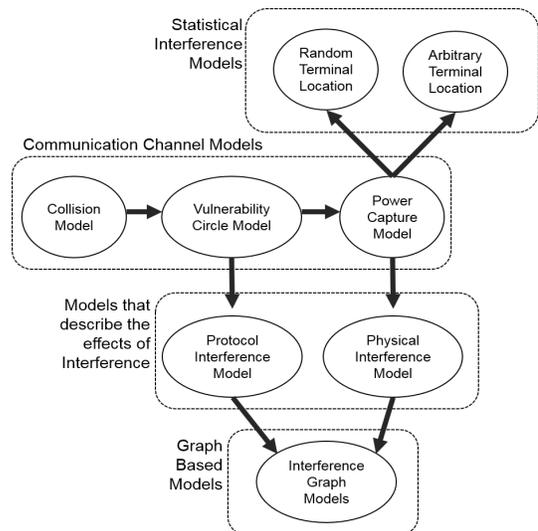
Figure 3: Unified view of interference models shown in [18]
