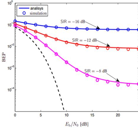
**Figure 4:** Bit error probability of BPSK versus  $E_b/N_0$  in the presence of the cognitive network interference.  $\lambda = 0.1 \text{ users/m}^2$  and  $\zeta = 40 \text{ dBm}$ . For comparison, the BEP in the without interference is also plotted (dashed line).
