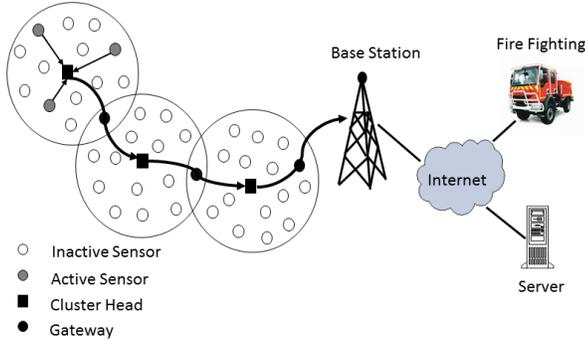
**Figure 1. The proposed architecture for forest fire detection.**
