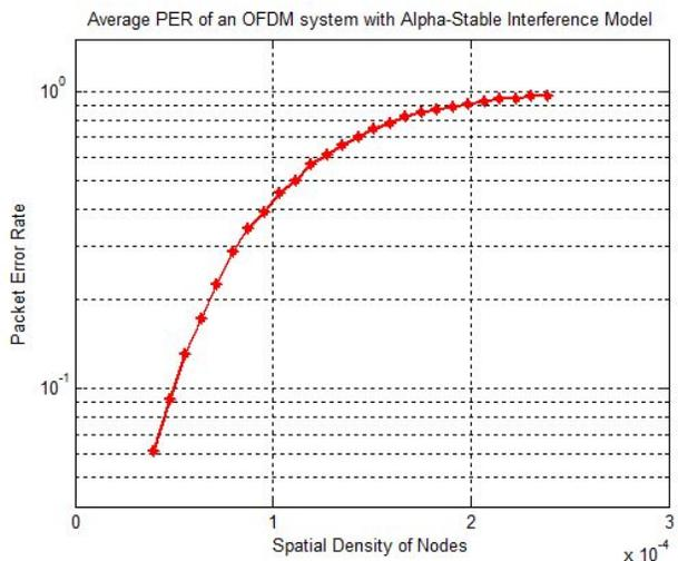
Figure 3. PER performance of PHY layer based on OFDM with alpha-stable interference model.
