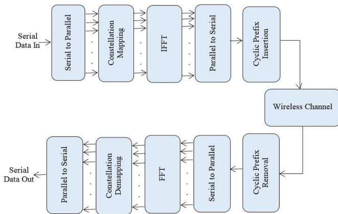
Figure 1. Block diagram of OFDM based Transceiver.
