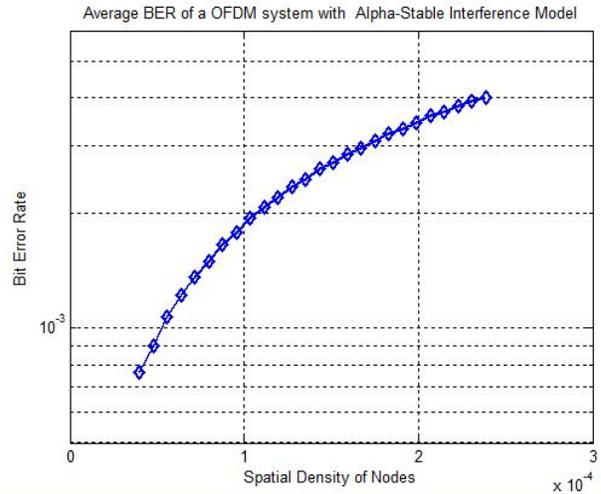
Figure 2. BER performance of PHY layer based on OFDM with alpha-stable interference model.
