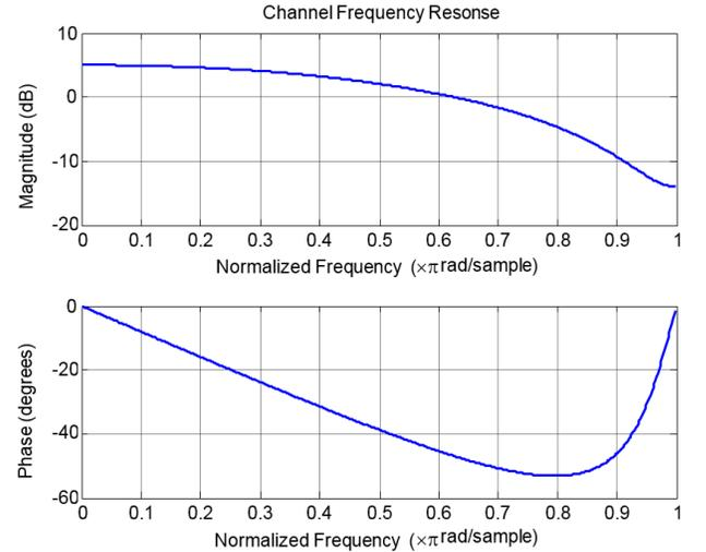
Figure 8. Channel frequency response for [1 0.8].
