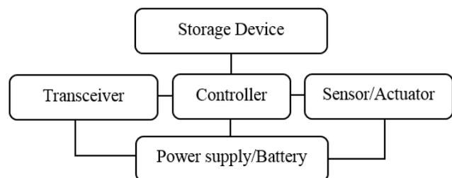
Figure 1. Basic architecture of a sensor node.
