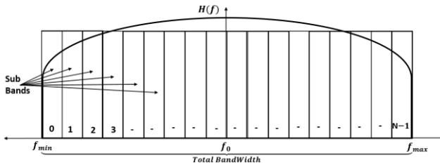
Figure 5. Ground concept of OFDM.
