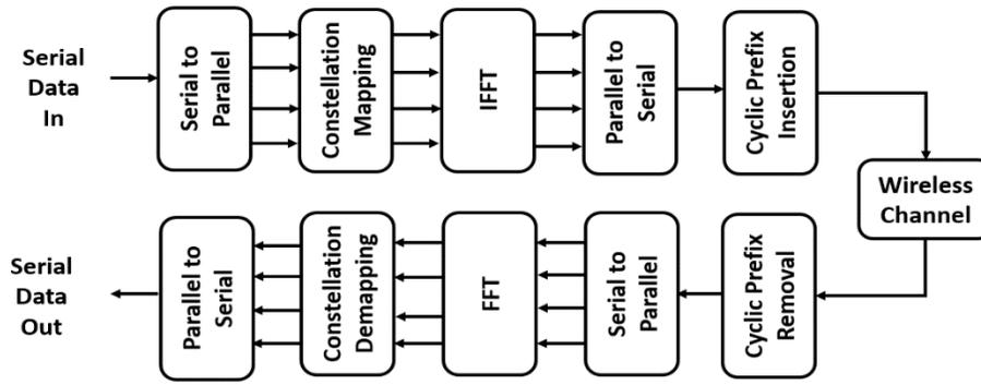
Figure 4. Functional Block Diagram of an OFDM Communication System.
